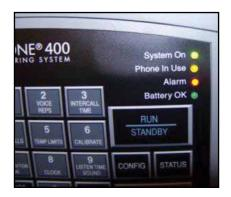
When feed drops away from the Bin Flag, the rotator will change from yellow to black. This will also trigger an alarm condition and the indictor light next to Alarm LED will blink red. The unit will also begin its call out procedure alerting the call list of the feed outage condition.
