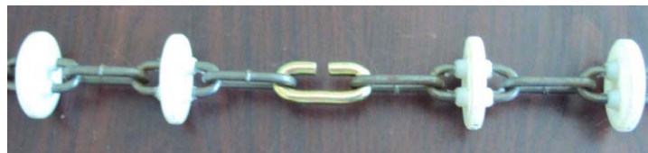
Incorrect way to connect chain to Coupler
