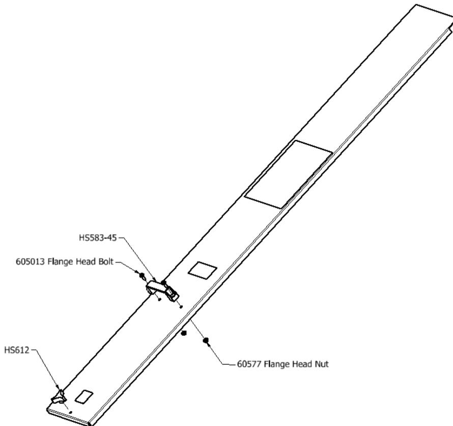
**HS612 Tri-Handle Knob installs over threaded stud when cabinet door is placed on machine.**
