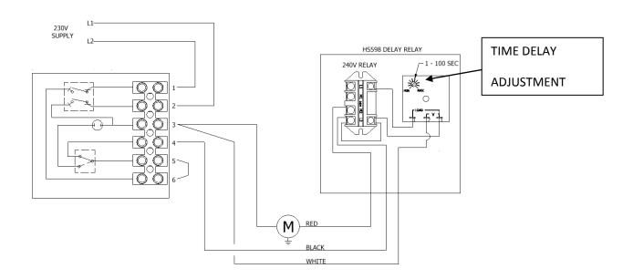
Wiring for use with GrowerSELECT HS593 Control unit or CTB 6500 Control Unit
