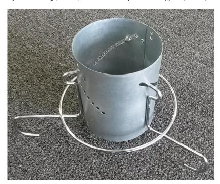
5. Drop the feed tube (Item 5) into the assembly as shown.
