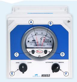
**A** Pressure reading drops below this limit, the vent machine **CLOSES** vents to raise the pressure inside.
