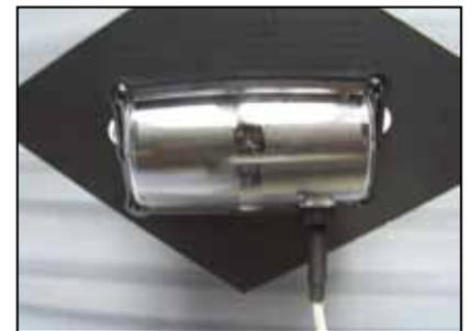
When feed drops away from the Bin Flag, the rotator will change from yellow to black. This will also trigger an alarm condition and the indicator light on the panel will turn red. The unit will also begin its call out procedure alerting the call list of the feed outage condition.
