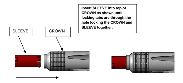
Install assembled CROWN and SLEEVE onto HS577 KWIKSTART outlet tube.
